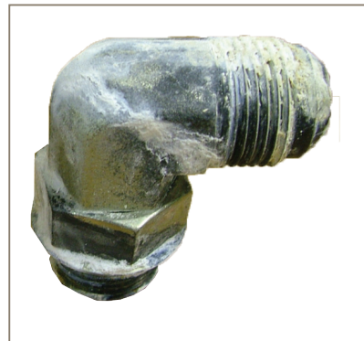
Figure 5: Zinc Oxidation on a Steel Tube Fitting
